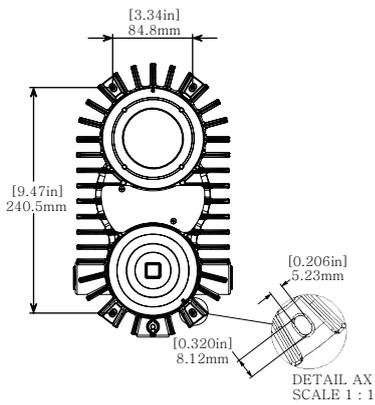
Mounting tabs sized for M5 or #10 fasteners.
